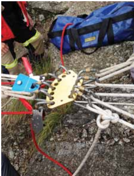
Floating anchor as constructed by Durban University of Technology
